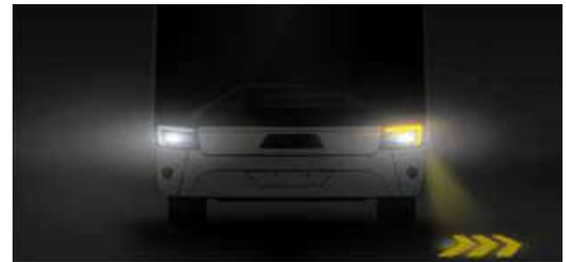
Left-turn Signal Projected on the Ground to Enhance Safety
